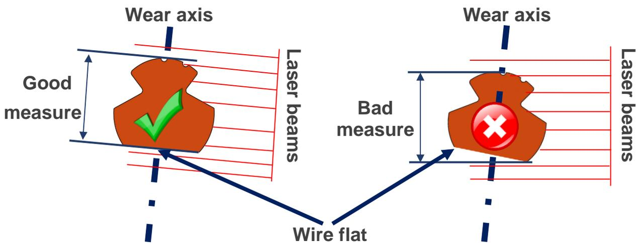
1. After placing the device on the contact wire, press the "Reset Flat" button.
