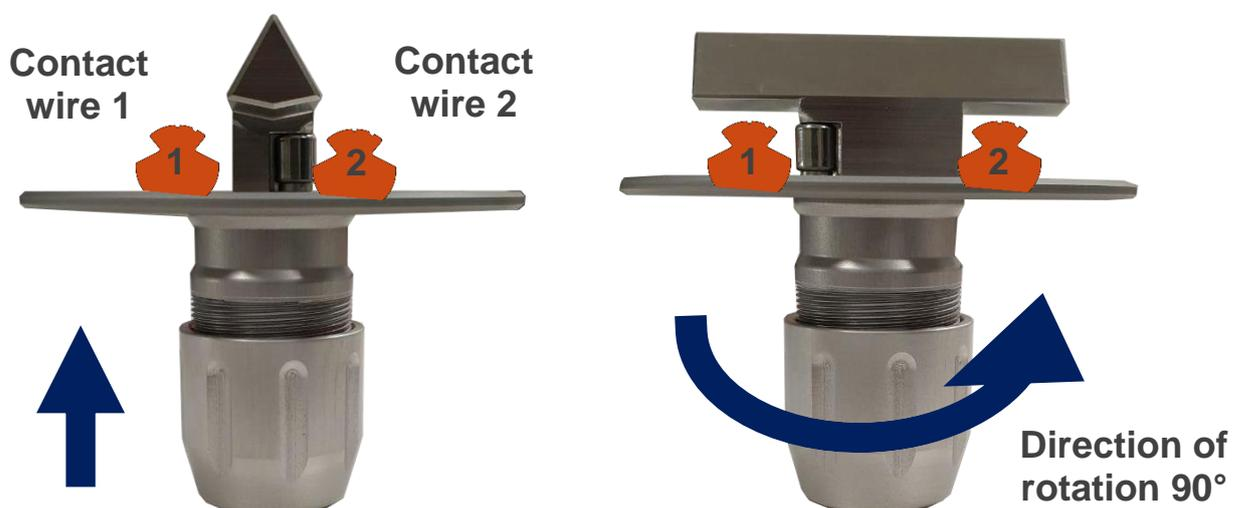
**!** The direction of rotation is represented by the arrows visible on the spreader.
