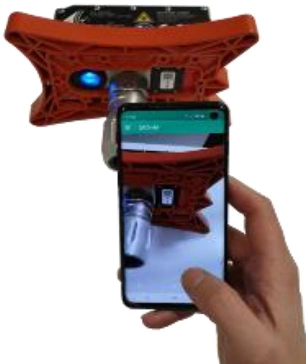
4. The app is connected to the tool if the app recognizes your tool's serial number and the color bar changes to green.
