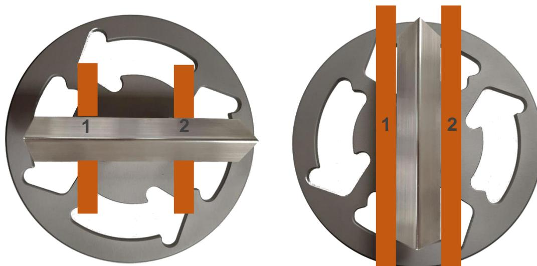
**!** The direction of rotation must be the opposite of that represented by the arrows of the spreader.
